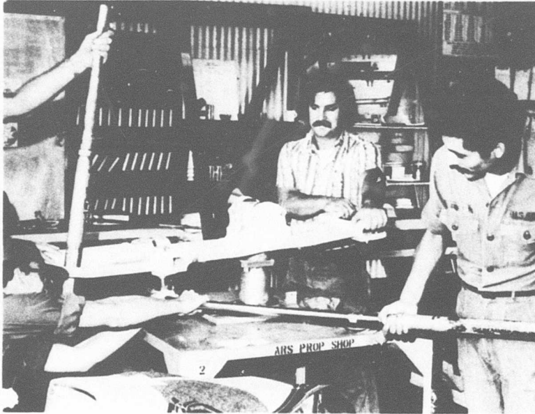
Figure 40. Removal of extension-to-yoke attach bolts, AH-1 main rotor hub.
