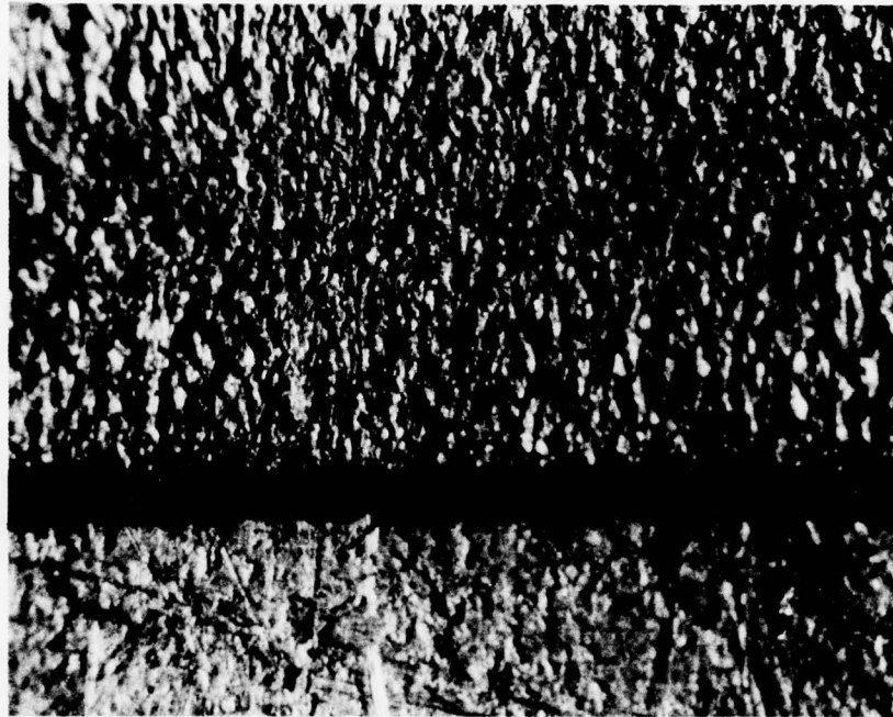
Figure 14. Surface appearance before and after low temperature cycling of 45 v/o, 0.045 thick 6061 Al-B.
