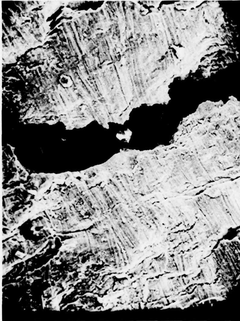
Figure 17. Crack in surface of thermally cycled longitudinal carbon-2024 aluminum at a magnification of 350.
