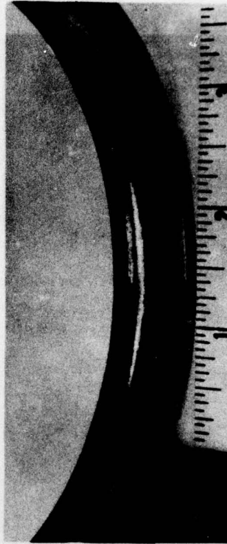
SPALLED OUTER RACE
