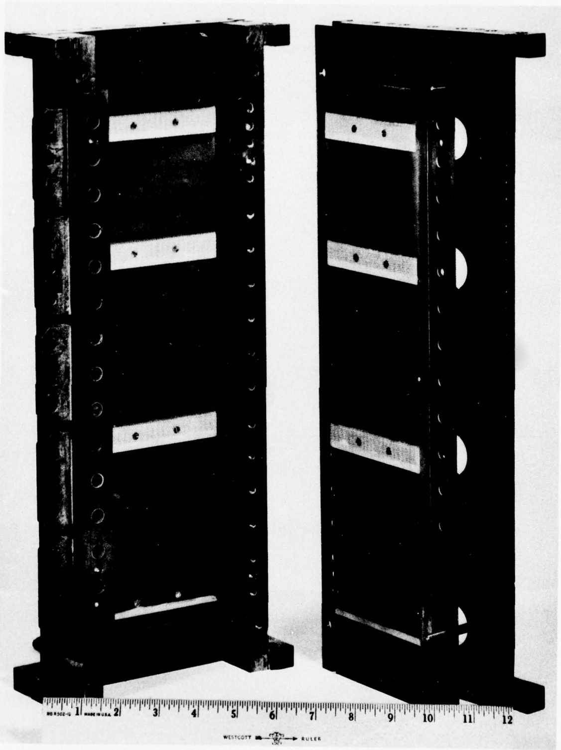
Figure II.3. Disassembled Diverging Channel II
