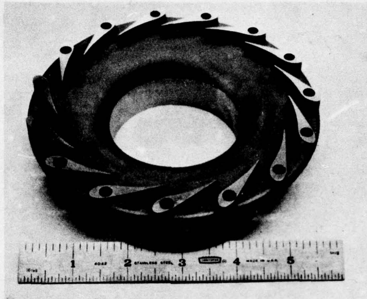
STANDARD 10 kW REAR NOZZLE SHROUD (Part #107726-1) (Turbine Seal Surface Not Machined)
