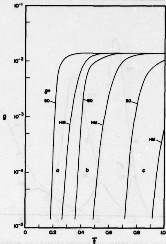
FIG. 15-a TIME-VARIATION OF CONDENSATE MASS FRACTION ALONG PARTICLE PATHS INITIALLY AT -5(a), -10(b), -20(c), cm THE DIAPHRAGM
