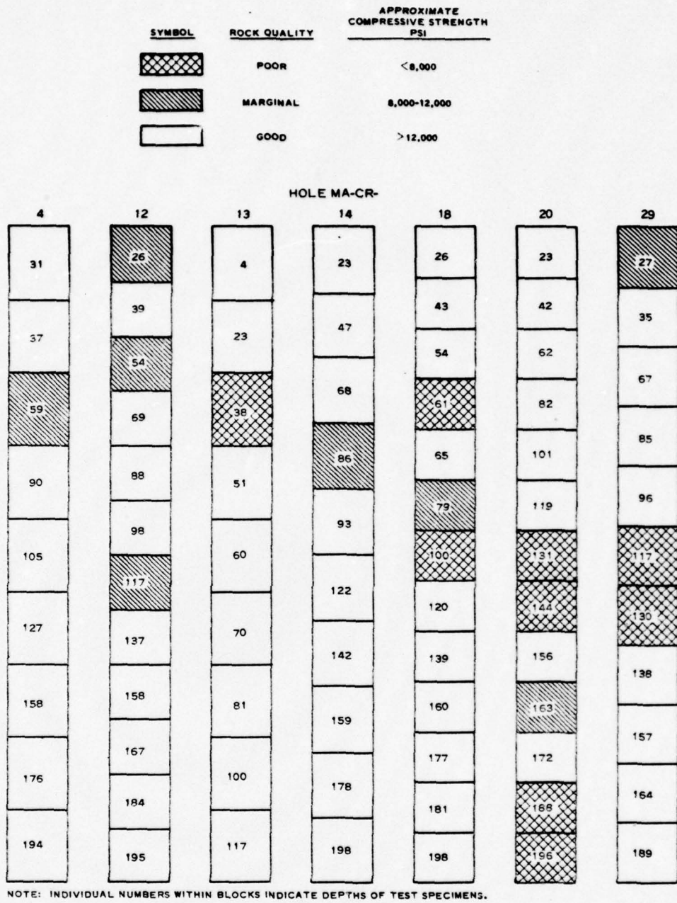
Figure 5.1 Depth versus quality for individual holes.
