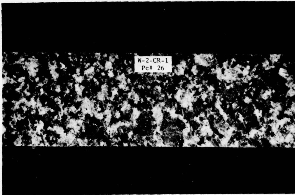
Figure 4.1 Granite specimen, Core W2-CR-1, Section 26, showing typical porphyritic texture of the granites from the Warren II area. White specks near the black biotite are kaolinite. The large fractured grains are phenocrysts of microcline.
