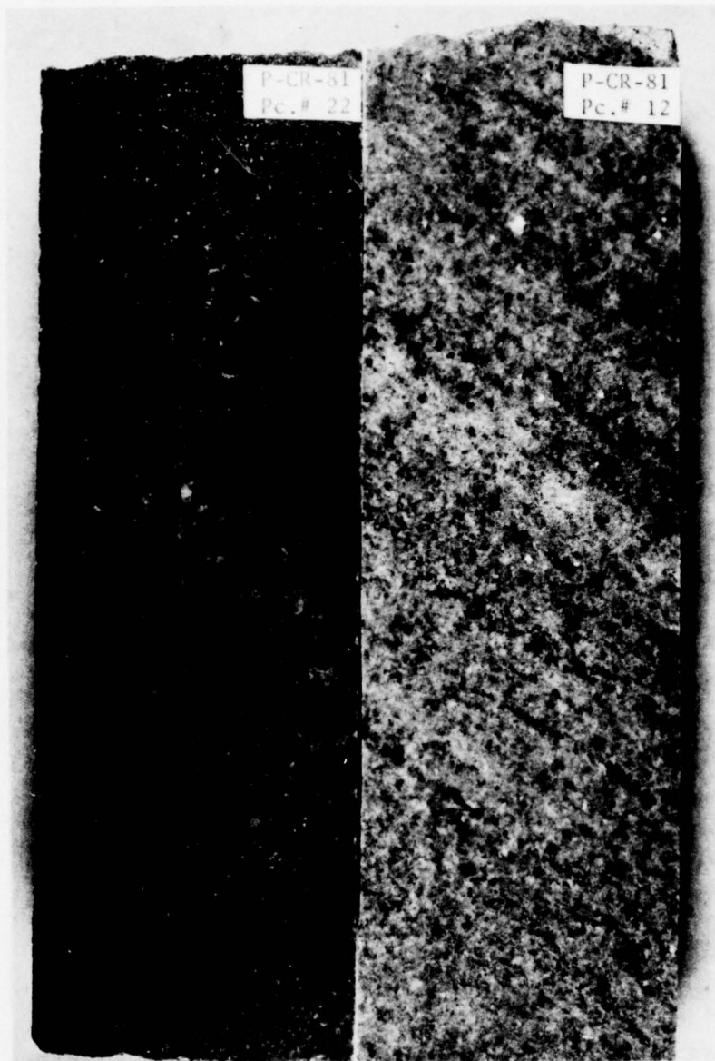
Figure 4.5 Gneiss sections, Core P-CR-81. Section 22 shows medium-grained texture and lack of foliation. Small white specks are magnetite. Section 12 shows grain size similar to 22 but has well developed foliation.
