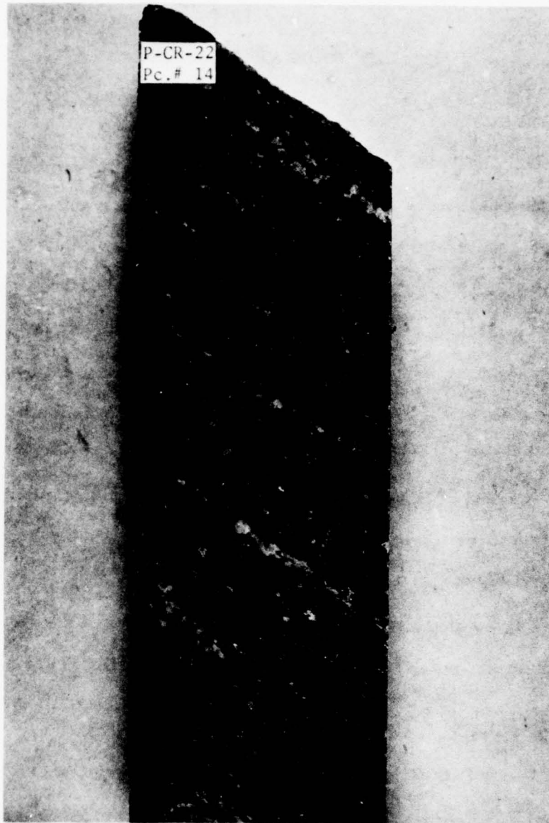
Figure 4.7 Amphibolite section, Core P-CR-22. Section 14 shows well developed foliation due to parallel alinement of hornblende and biotite.
