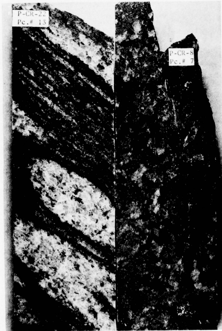
Figure 4.3 Gneiss sections, Cores P-CR-8 and P-CR-22. Section 13 shows large white augen of quartz, plagioclase, and microcline elongated parallel to the foliation. The foliation bends around the augen. Section 7 shows several fractures (narrow white and black lines) and pyrite introduced along the fractures (white specks near top and bottom).
