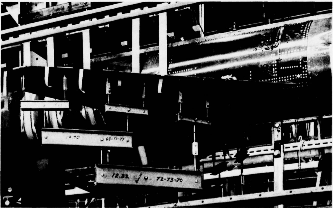
Figure 10-2: XBQM-34E Wing Loading System
