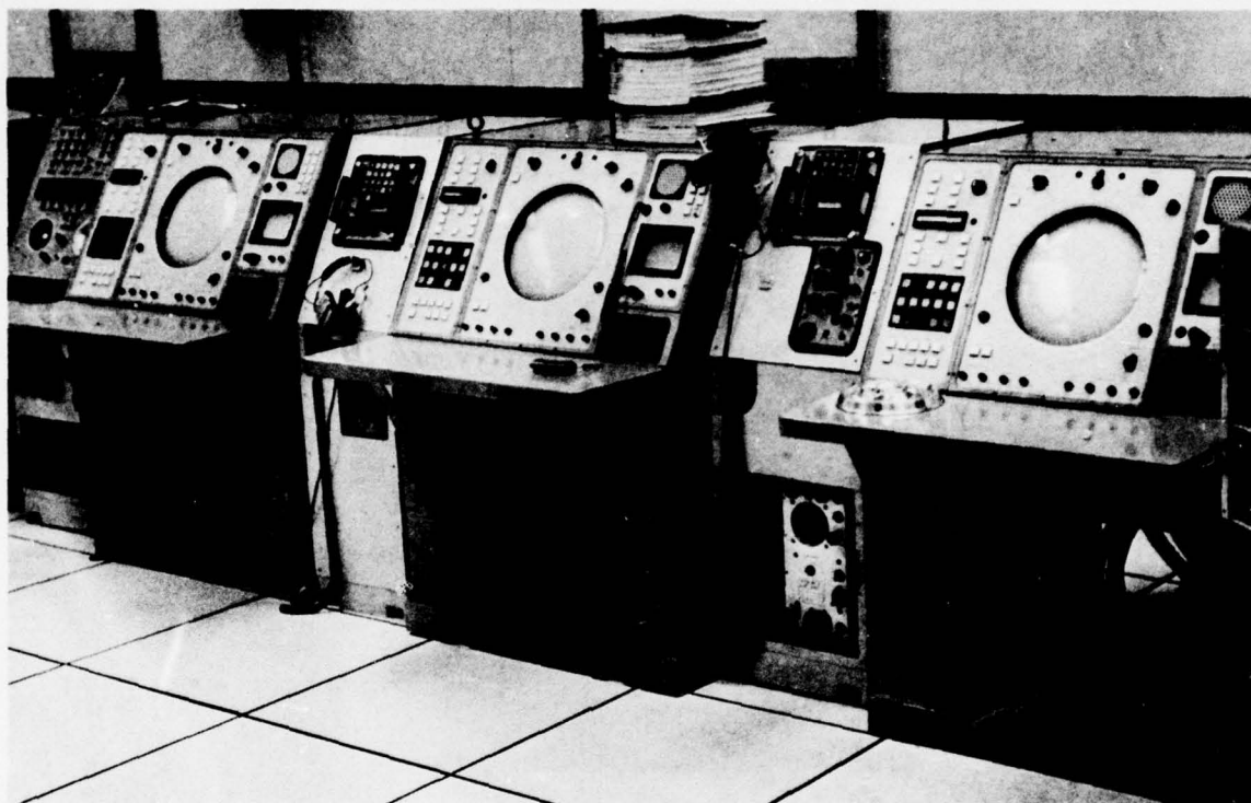
Figure 3. Situation Display Consoles. Three Situation Display Consoles located at the Canadian Forces Fleet School are shown. The consoles have 12" diameter and 5" (diagonal) cathode ray tubes.
