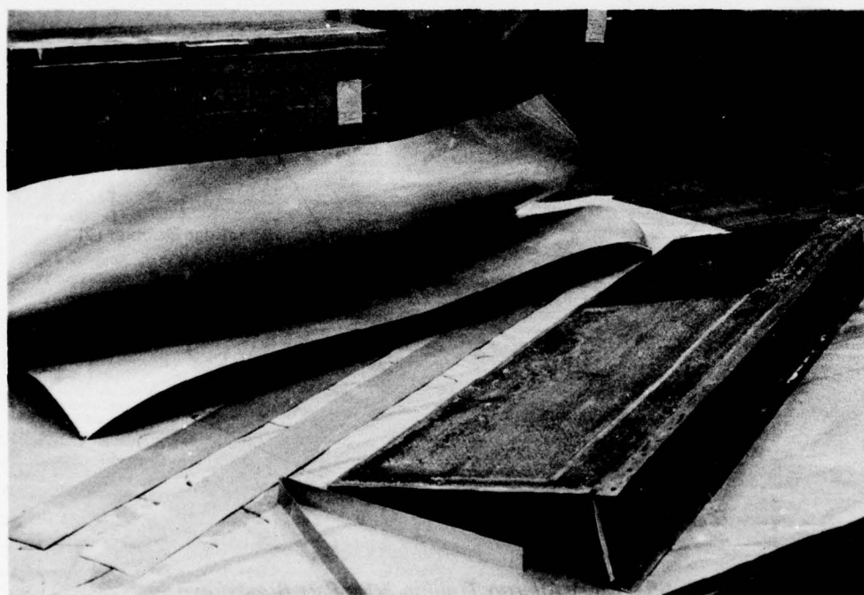
Figure 67.—C5-A Aileron Trailing Edge Repair Details Ready for Bonding
