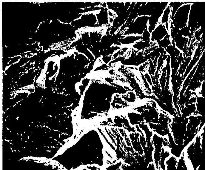
Figure 23. Cleavage facets in an A-588 Charpy specimen tested at -196^{\circ}\text{C} , 1000X.
