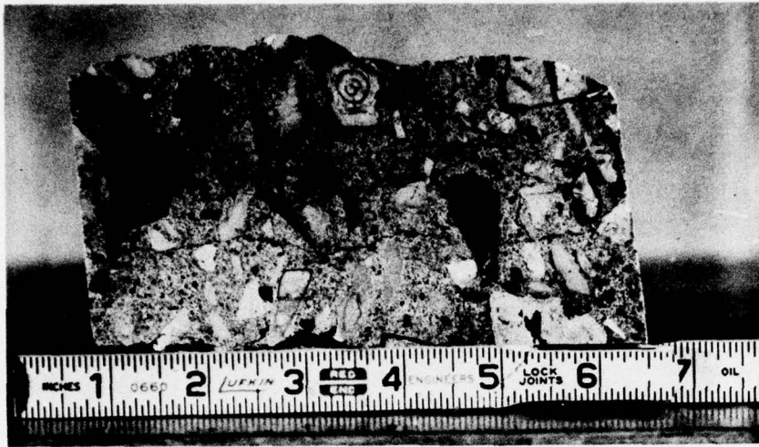
a. Sawed and ground surface of a portion of core 3 from an arch section. The aggregate particles showing dark rims are chert that have reacted in the alkali-silica reaction. About half normal size.
