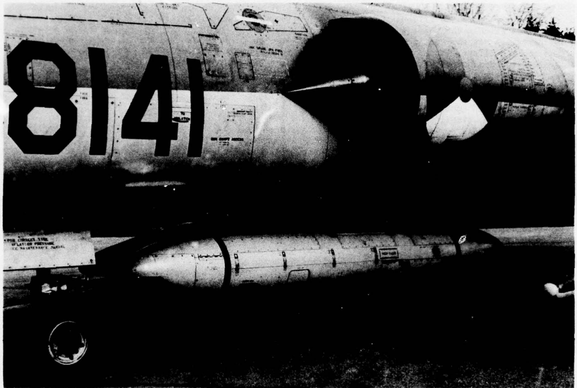
FIG. 1 ORPHEUS RECONNAISSANCE POD ATTACHED TO A LOCKHEED RF-104G
