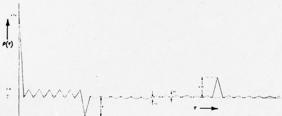
Figure 6.5 Autocorrelation of a 4-bit Barker Code each bit of which is a 13-bit Barker Code
