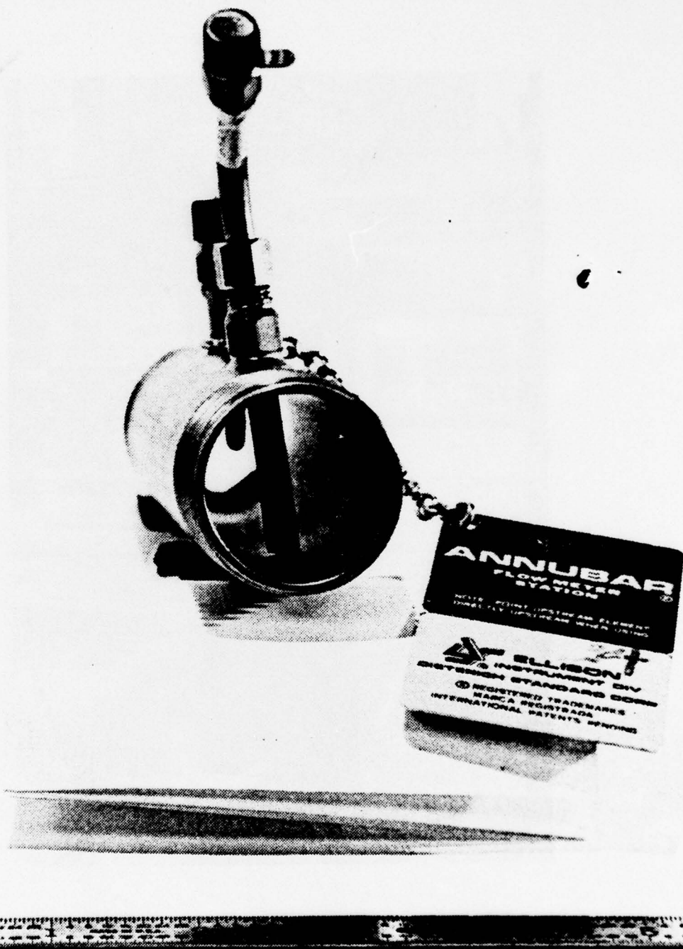
FIGURE 32. Photograph of the Annubar, Primary Flow Sensor.
