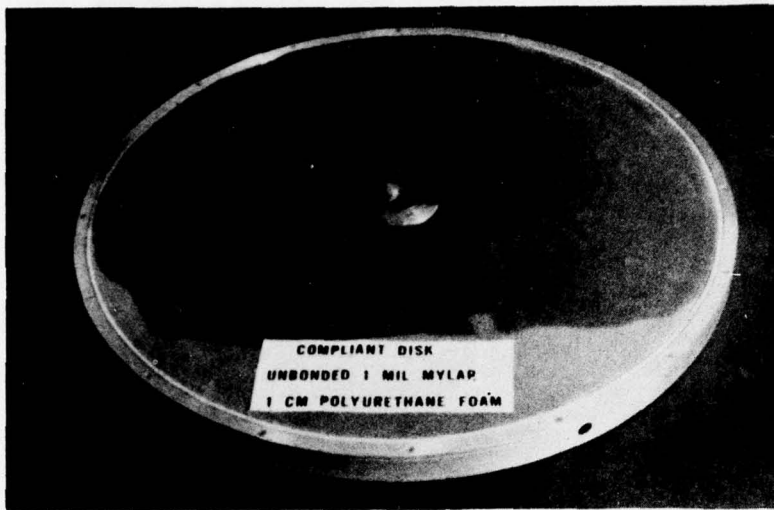
FIGURE 3-10. FINISHED COMPLIANT DISK
