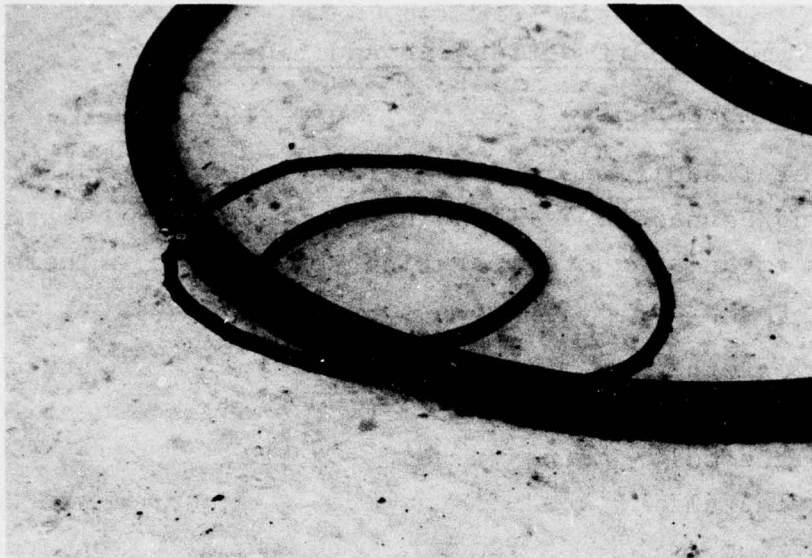
Figure #1: Cracking of Standard V-Belts After Low Temperature Testing
