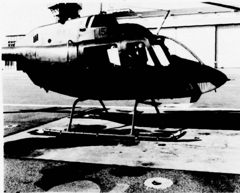
Fig. 1 High Tubular Skid Gear Kit and Snow Kit as Installed on the Model OH-58A Helicopter, BHC Photo No. 385277
