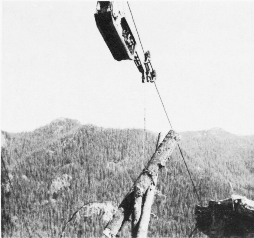
Logs being delivered downhill to the landing by a "sky car." This system also keeps timber free of the ground, holding ground disturbance to a minimum. (Forest Service)
