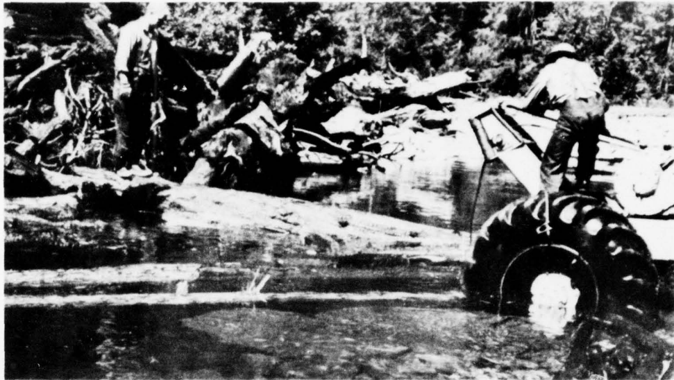
A rubber-tired tractor removes debris from an anadromous fish stream in the Coastal Subregion. (Forest Service)
