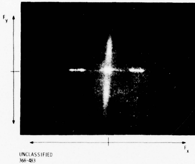
Figure 2-29. Two Dimensional Transform of a Single Dimensional Signal from an Accelerometer Output
