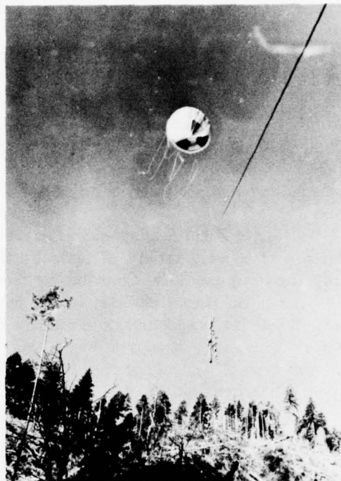
Balloon logging research aimed at reducing damage to surrounding area during harvest.
