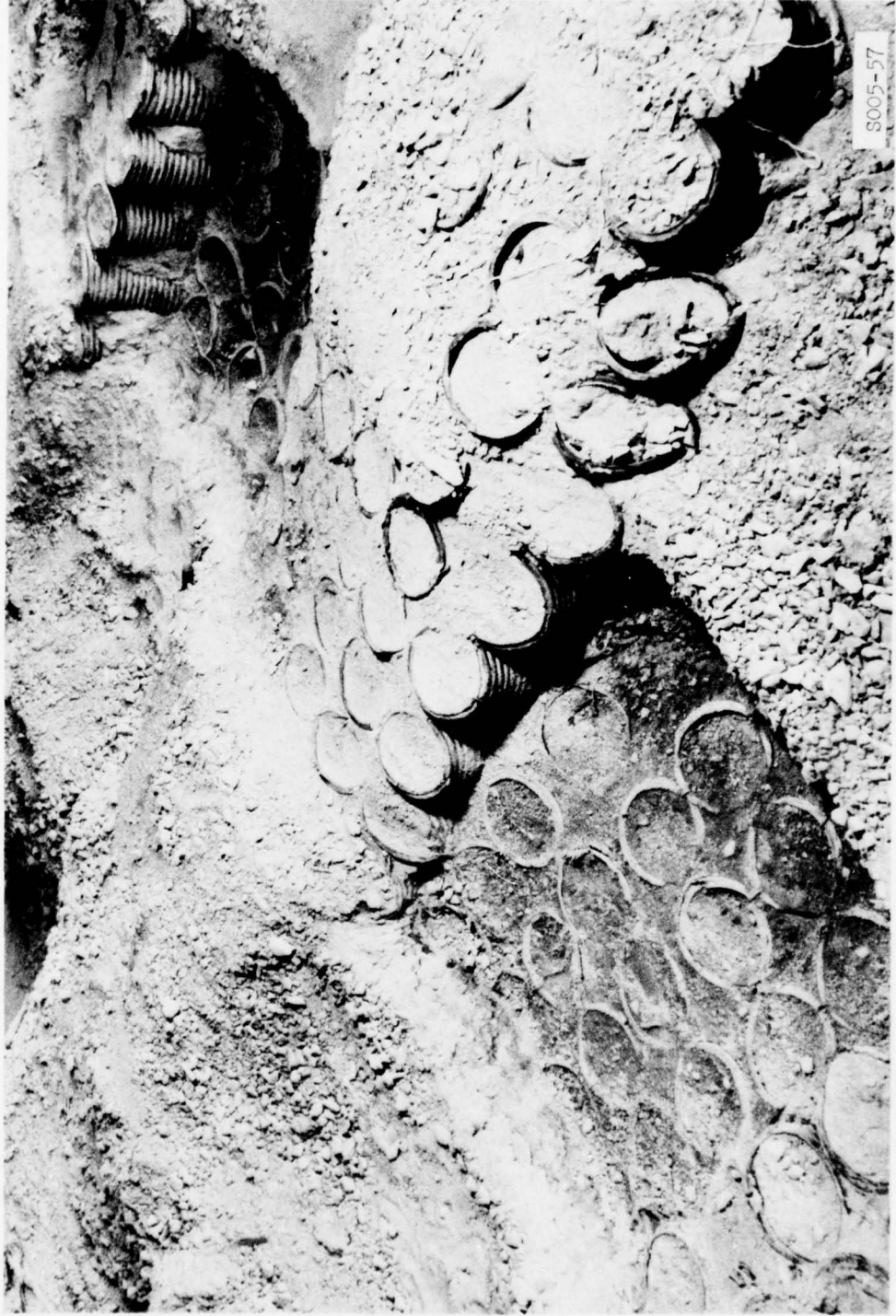
Photo 28. Item 4 with wearing surface removed after 5500 coverages
