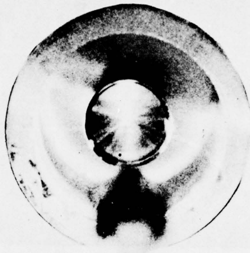
Figure 5. End view of discharge. Bright area on top is due to over-exposure of film by wire as viewed slightly downward. Note radial streamers characteristic of high-pressure discharges.
