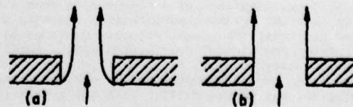
Fig. 2. Does the flow into the plenum chamber form a free jet inside the slot as in (a), or not, as in (b)?
