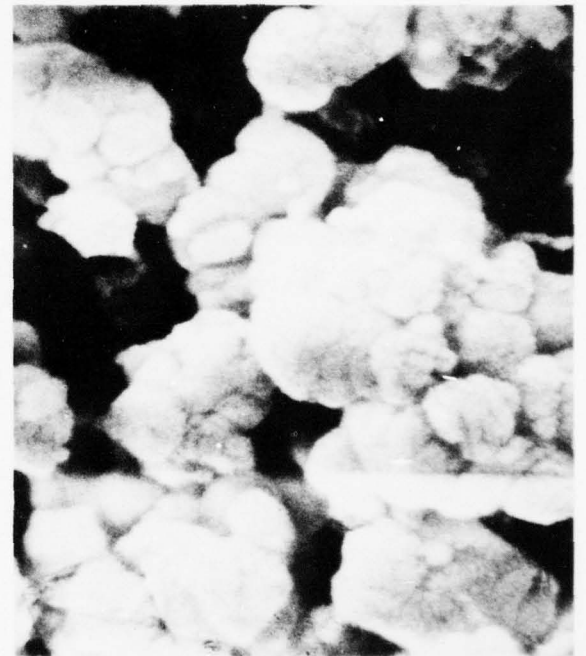
Figure 29(B). SEM Photo- micrograph of Microstructure of a Compact of SN-402 Si 3 N 4 Contain- ing 1 wt% B Fired at 1800°C for 30 Min in N 2 22,000 X
