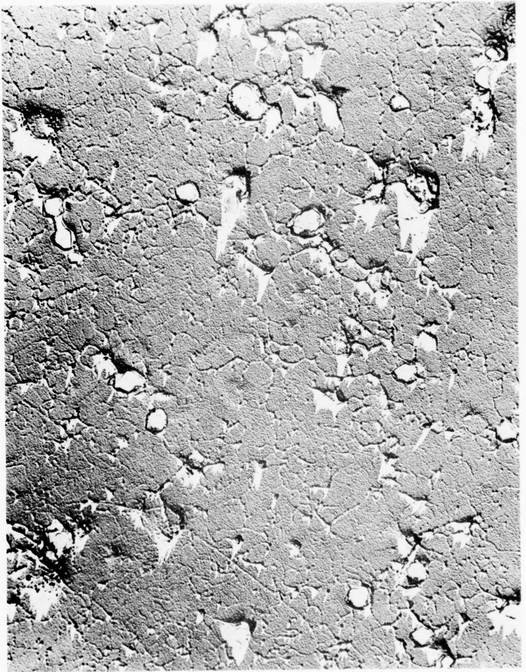
Figure 12. TEM of Replica of Polished and Etched Surface of Specimen No. 2 White Spots Correspond to Leached Out Silicon Grains. 30,000 X
