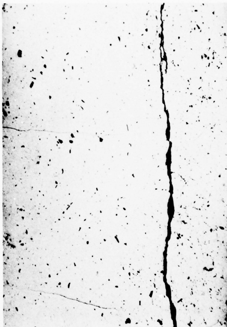
Figure 10. Section of a Typical \text{Si}_3\text{N}_4 Specimen Compacted at 5 GPa and 1500^\circ\text{C}
