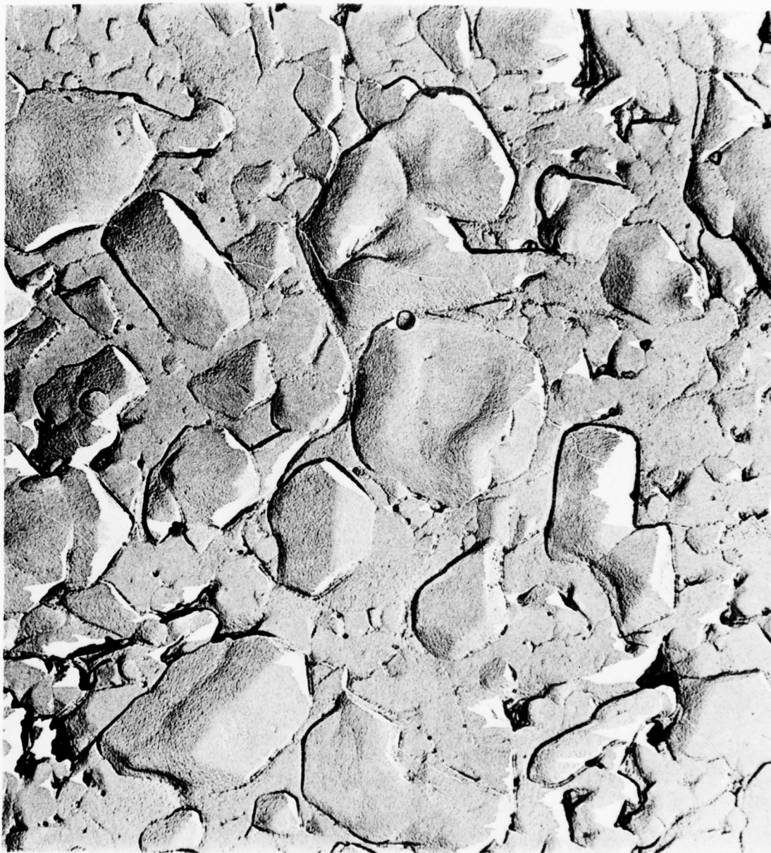
Figure 14. Microstructure of Poorly Bonded, Hot-Pressed \text{Si}_3\text{N}_4 (Specimen 5) TEM, Double Stage Replica 30,000 X
