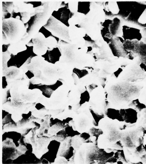
Figure 23. SEM Photomicrograph of Fractured Surface of Si 3 N 4 Prepared in Table 1, Exp. No. 3 Mag = 2000 X
