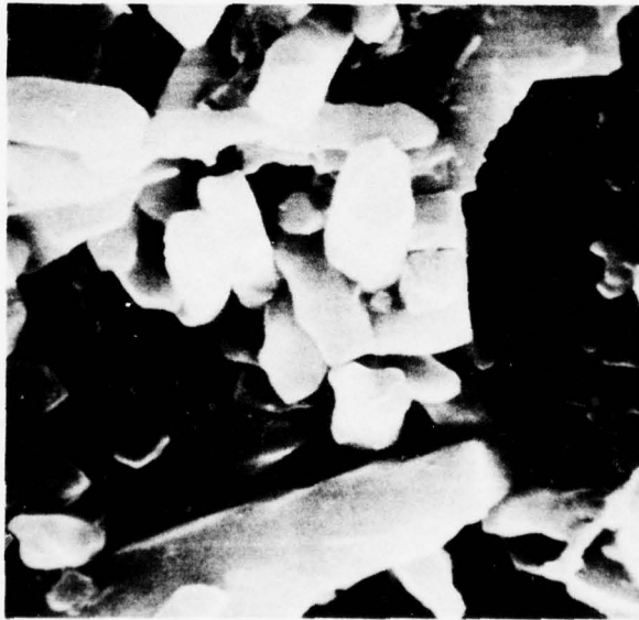
Figure 37. Morphology of Grains in \text{Si}_3\text{N}_4 Sintered at 2000^\circ\text{C} SEM, 10,000 X
