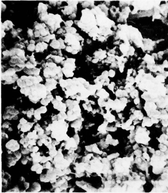
Figure 29(A). SEM Photo- micrograph of Microstructure of a Compact of SN-402 Si 3 N 4 Contain- ing 1 wt% B Fired at 1800°C for 30 Min in N 2 5500 X
