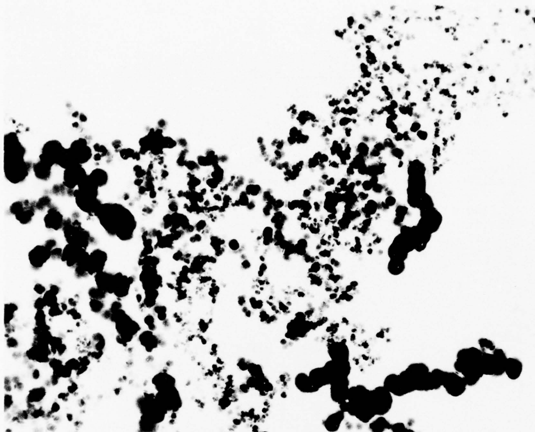
Figure 7. Particle Morphology of Amorphous \text{Si}_3\text{N}_4 Synthesized at 850^\circ\text{C} . 30,000 X, TEM
