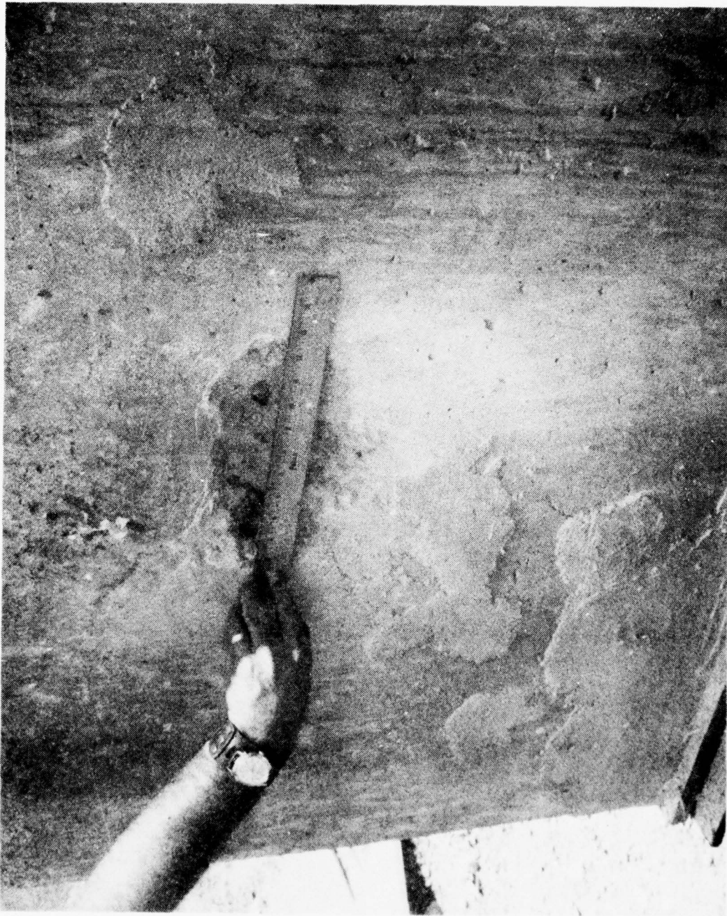
Figure 15. Test No. 15, Concrete Target Closeup with Residue Removed
