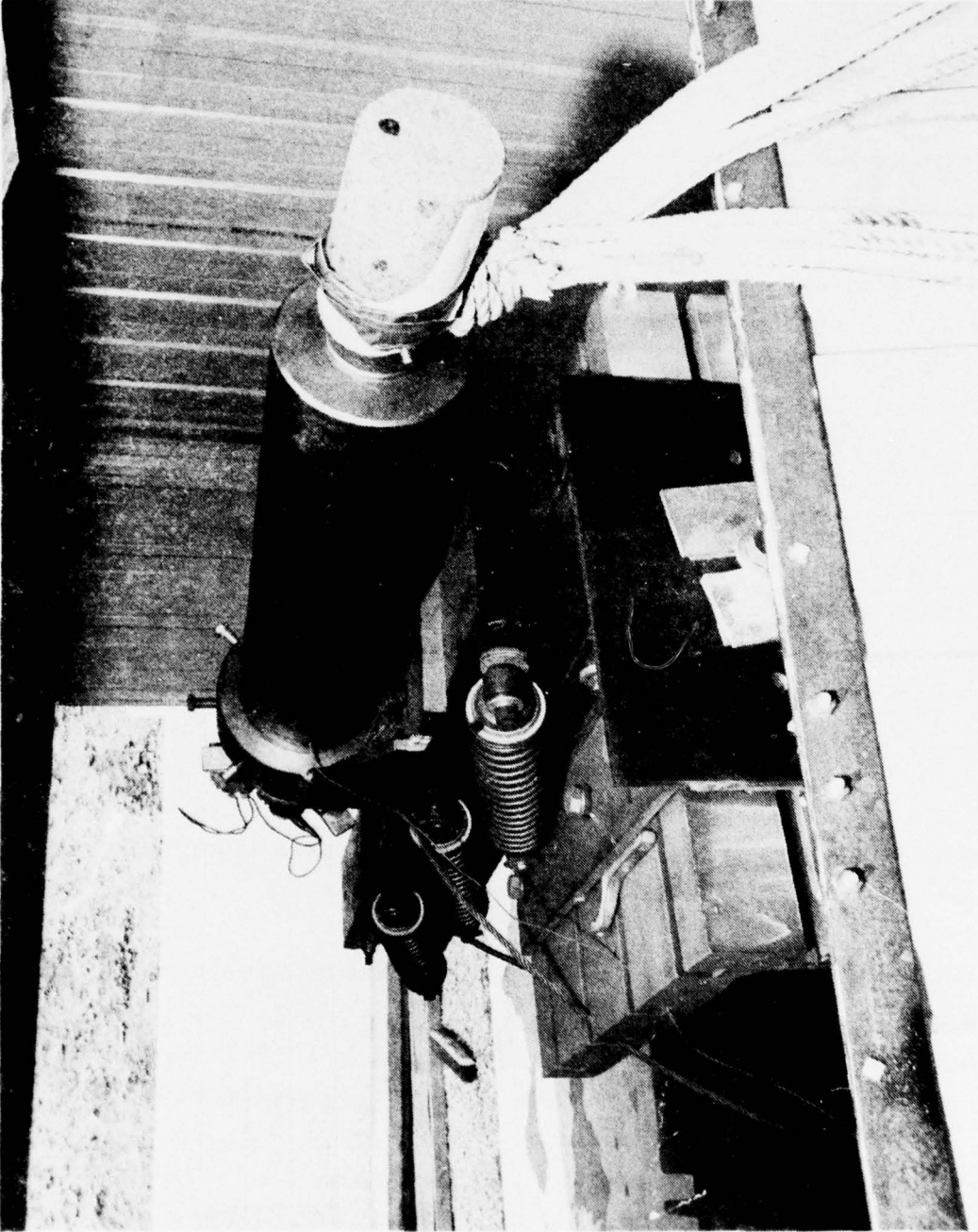
Figure 1. Rock Mortar - Front View with 10-lb Granite Projectile
