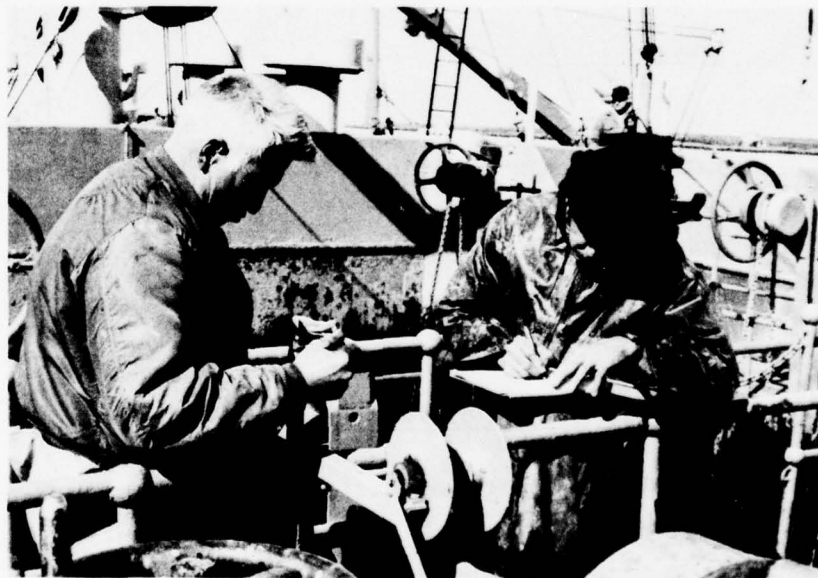
Figure 3-2. Making Torque Vane Measurements on the Hopper Dredge
