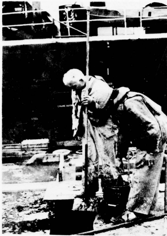
Figure 3-3. Penetration Tests Using a 1 sq ft Plate
