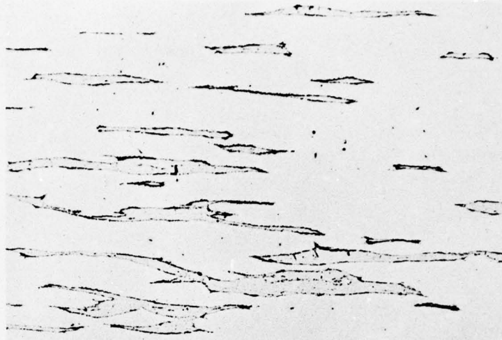
Figure 11. Photomicrograph of Billet #4 ( 90^{\text{V}}/\text{oTi}-10^{\text{V}}/\text{oBe} ) After Back-Extrusion - Bottom of Cup.
