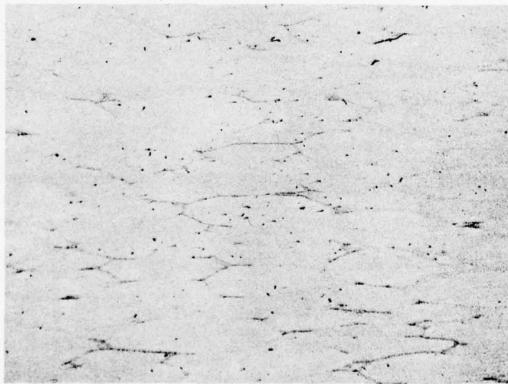
Figure 8. Photomicrograph of Billet #3 (100 V /oTi) After Back-Extrusion - Bottom of Cups.
