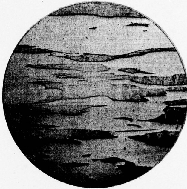
Figure 9. 70 V /o 7075 - 30 V /o ZK60A Extruded at 212°F. R = 6:1 Longitudinal
