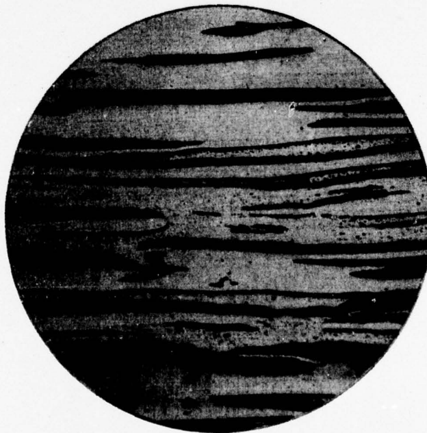
Figure 9. 70 V /o 7075 - 30 V /o ZK60A Extruded at 212°F. R = 6:1 Longitudinal
