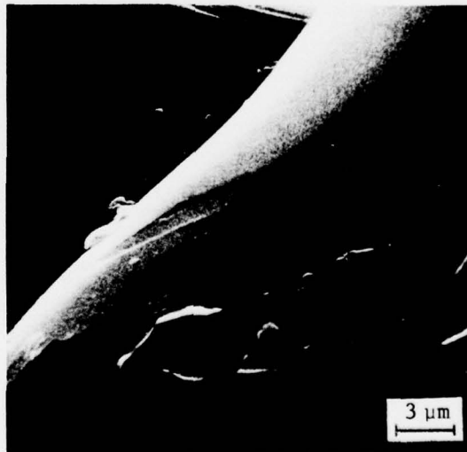
(b) Grain associated with initial flaw, showing apparent twin-induced microfracture
