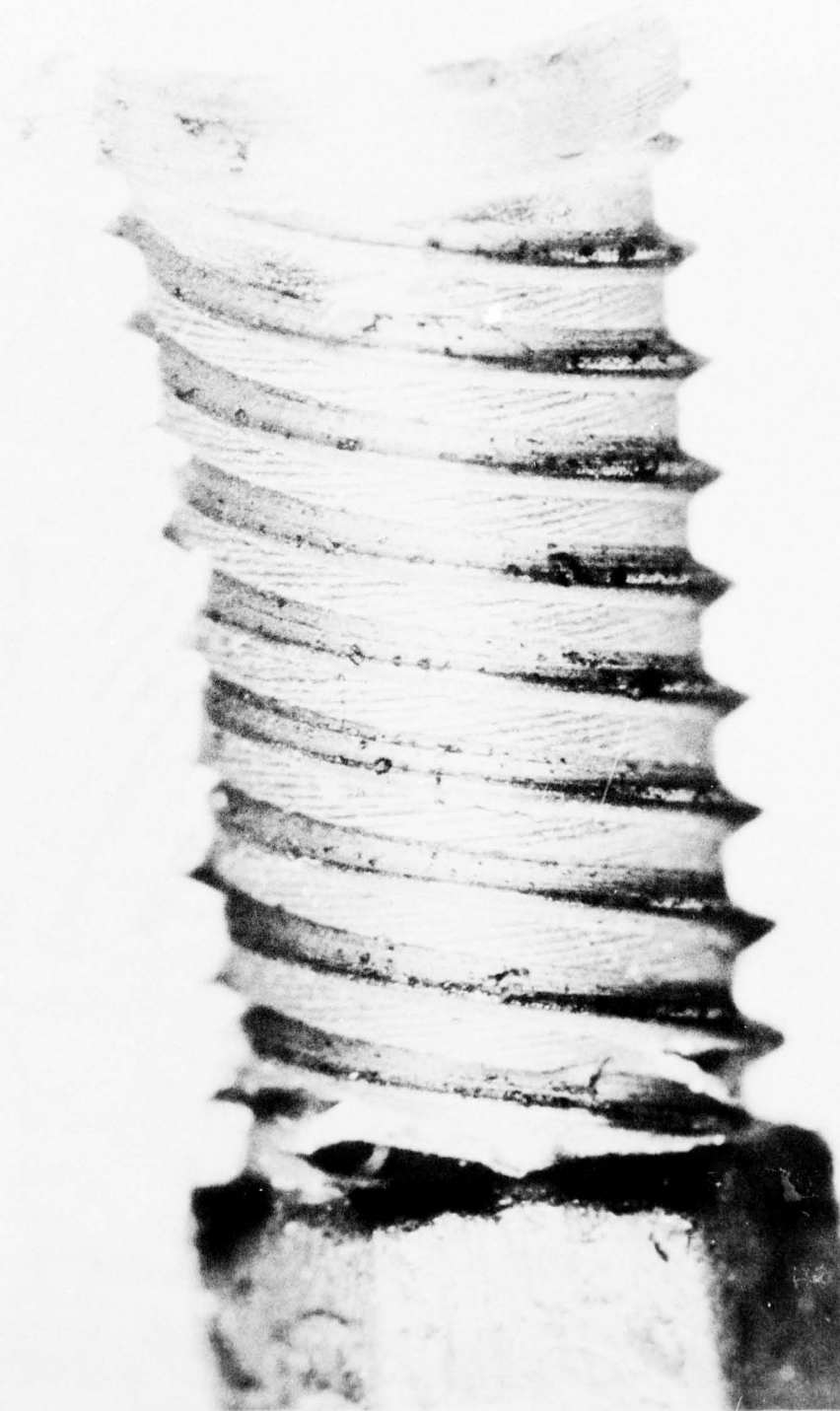
Figure 21. Truncated Thread Form From Failed Stud
