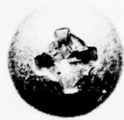
DRIVE RECESS FAILS
