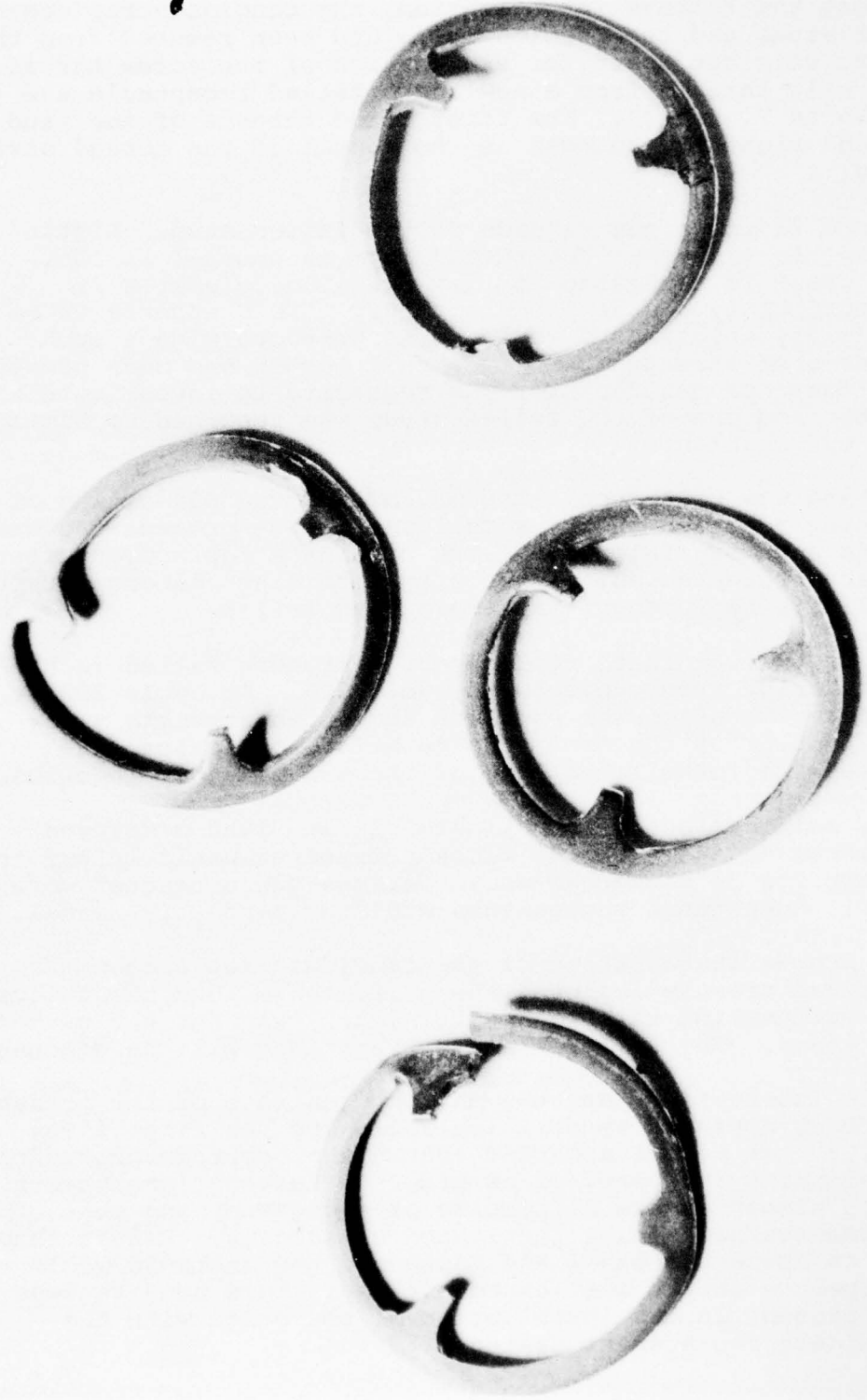
Figure 19. Candidate Replacement Stud Retaining Washer Failure
