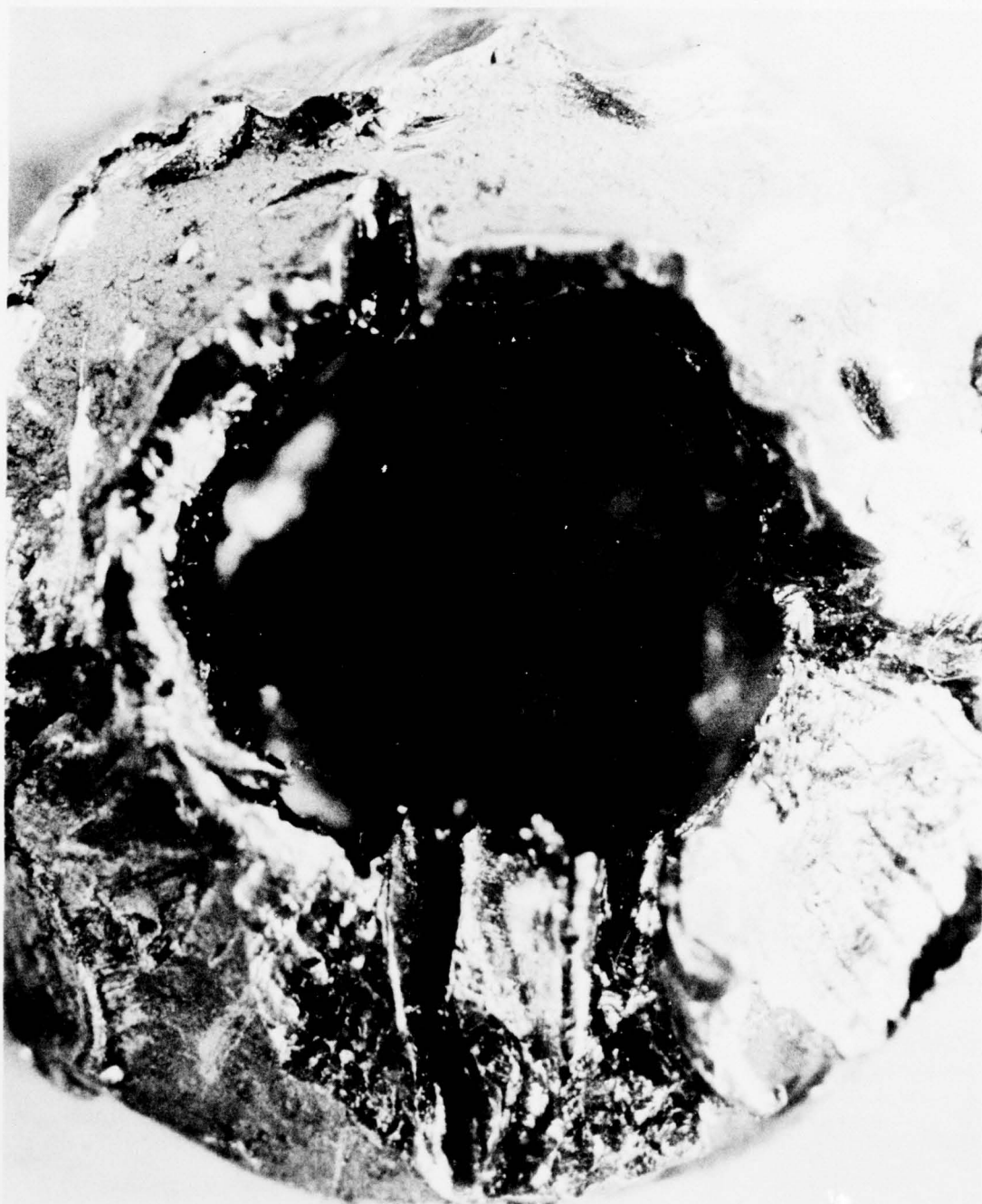
Figure B-6. Problems With Screw Removal After Recess Failure
