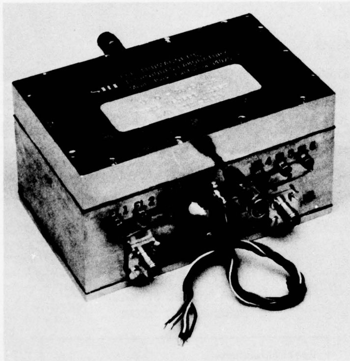
FIGURE A-1 K-BAND (18.0 to 26.5 GHz), MIC, IMAGE-REJECT MIXER, MODEL KIRM-2(2)
