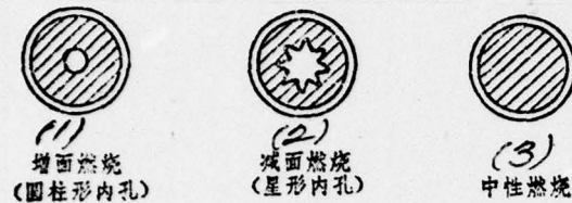
Fig. 5. Cross section configurations of three types of grains.
