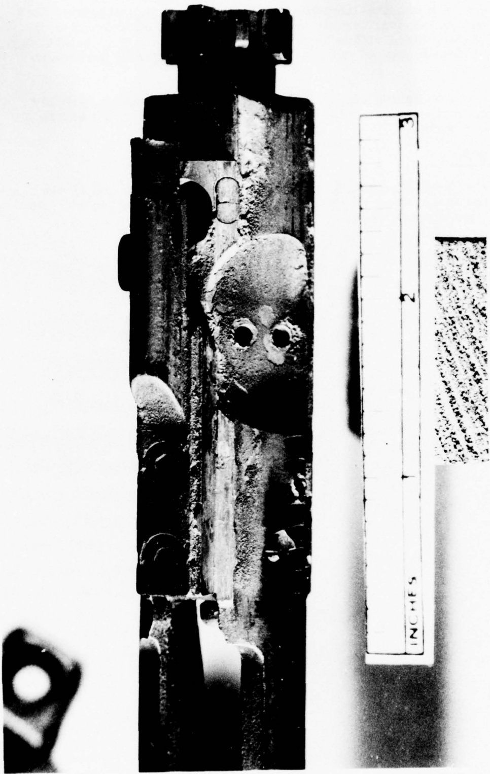
Figure 9. Bolt Carrier after 10,000 Rounds Showing Cracked Insert.
