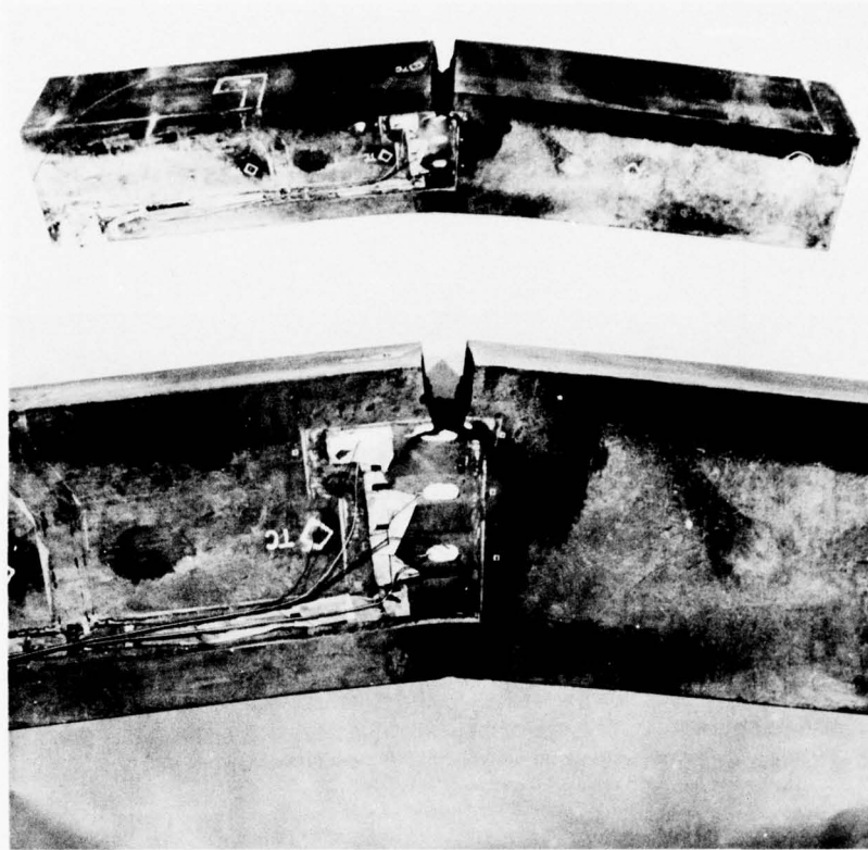
Fig. 96—Highly ductile performance of the 12-in. (300 mm) DT test specimen at 215°F (95°C). The size of the plastic enclave is indicated by the grossly dimpled region between the two tears that extend from the deformed crack root. The 750 000 ft-lb (104 000 kg-m) capacity of the equipment was insufficient to cause full fracture in this ductile mode.
