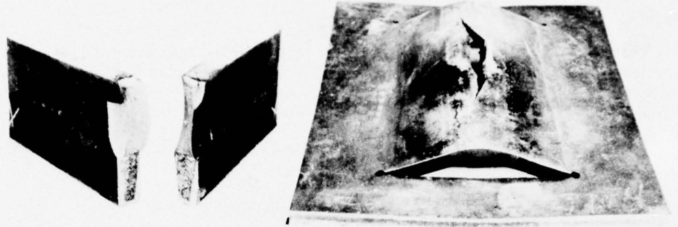
Fig. 104—Exact DT test reproduction of the characteristic fracture mode developed in explosion crack starter tests with through-thickness cracks.
