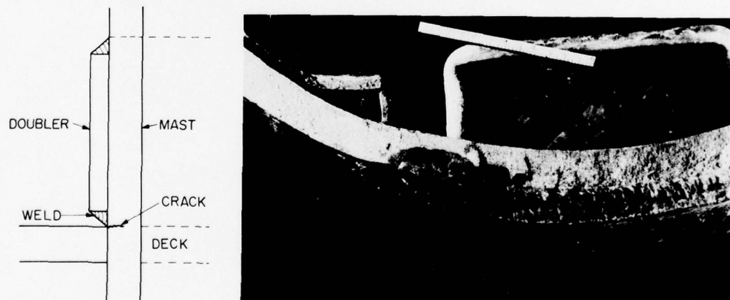
Fig. 1—Ship mast failure by brittle fracture.
