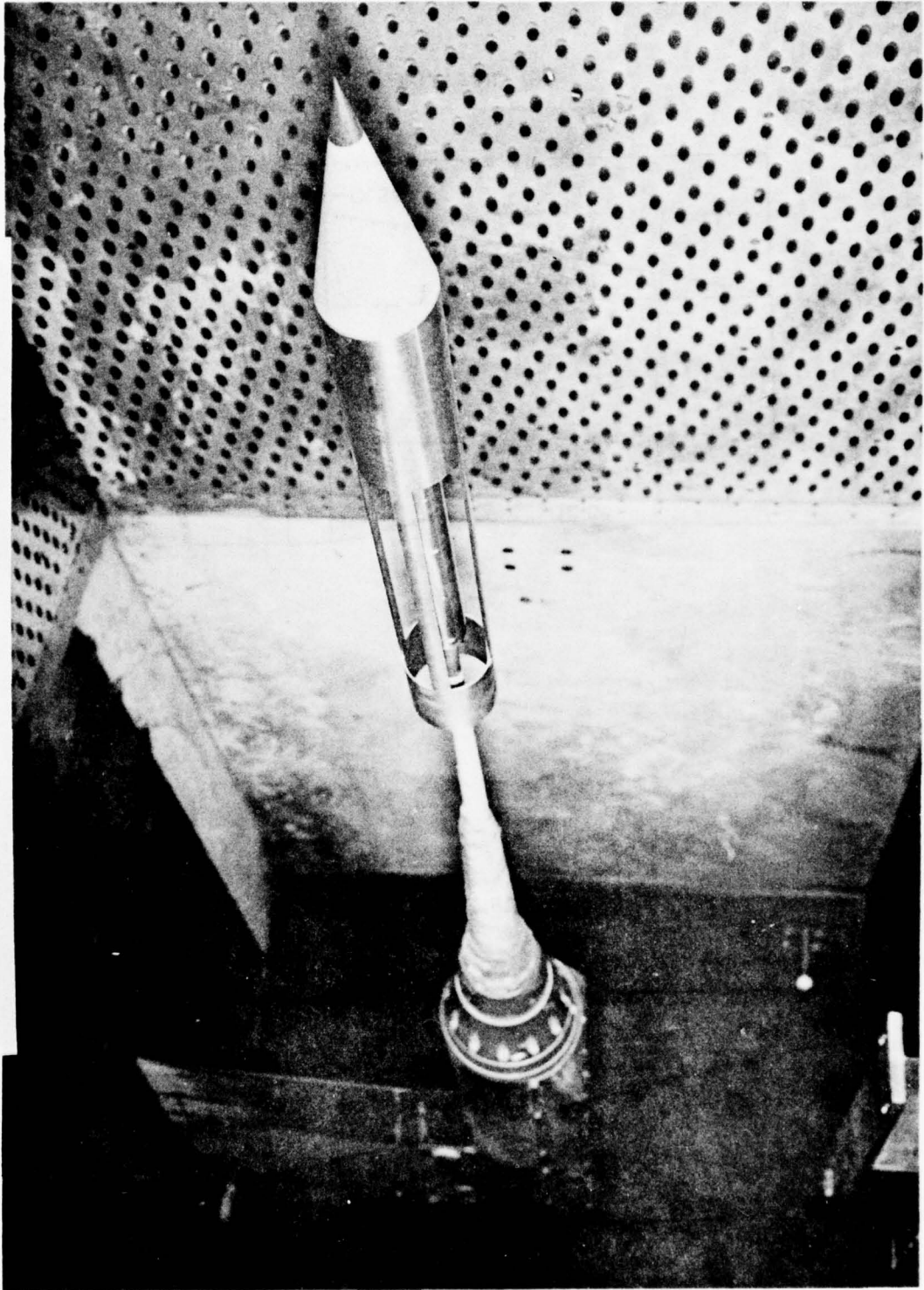
FIGURE 2. MODEL N 1 R 1 C 2 INSTALLED IN AEDC-PWT 4T WIND TUNNEL.
