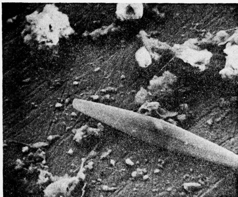
Plate 9.a. Stainless steel immersed 3 weeks, 500X. Solitary diatom.
