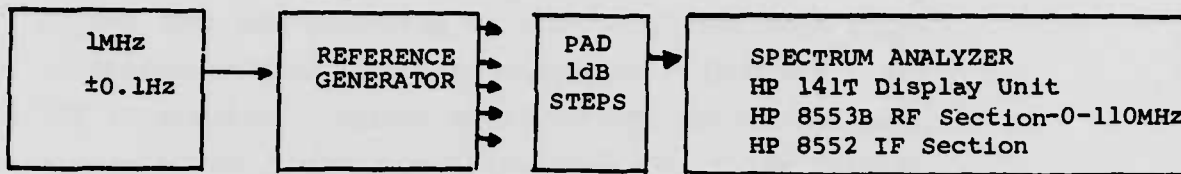
Figure 95. Reference Generator Spectral Purity Test, Bench Test Setup
