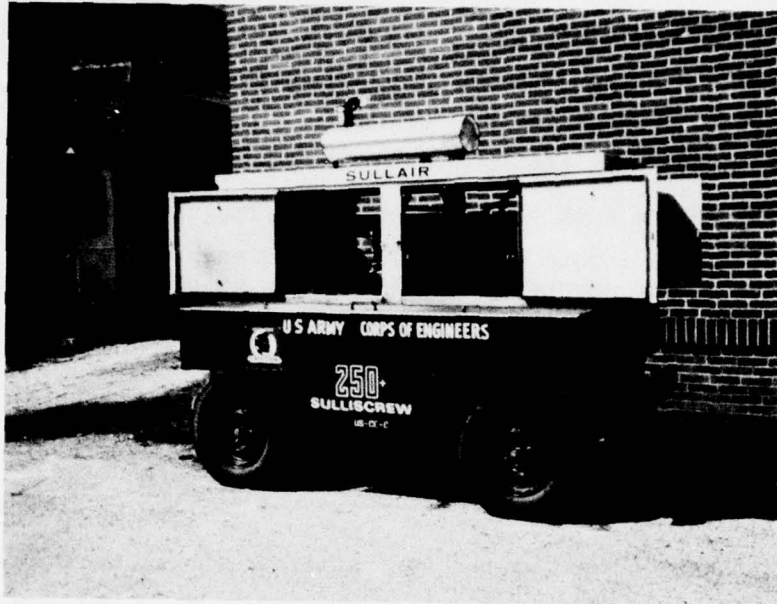
Figure 2. Sullair 250-cfm air compressor used for tests. Regulator set at 100 psi
