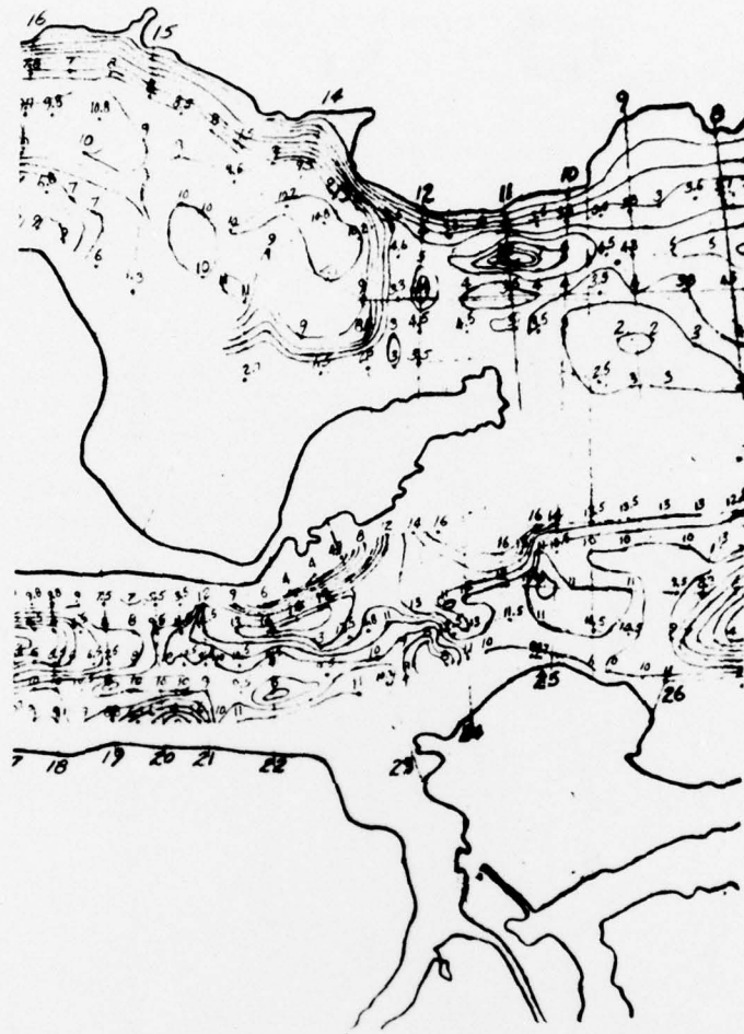
Figure 8. Contours drawn on the map from the ice thickness data.
