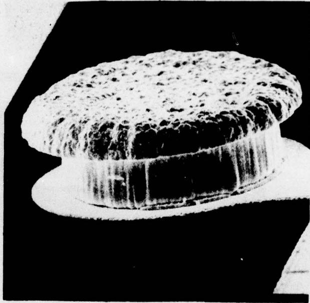
Fig. V-20 Cross section of a Au bond pad plated by means of the wet photoresist process.
