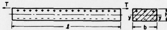
Freshly generated platelet with surface tension force acting on outer (old) surface only.
