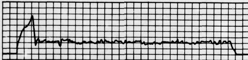
Typical chart recording of test data, single wheel "lock-up."
