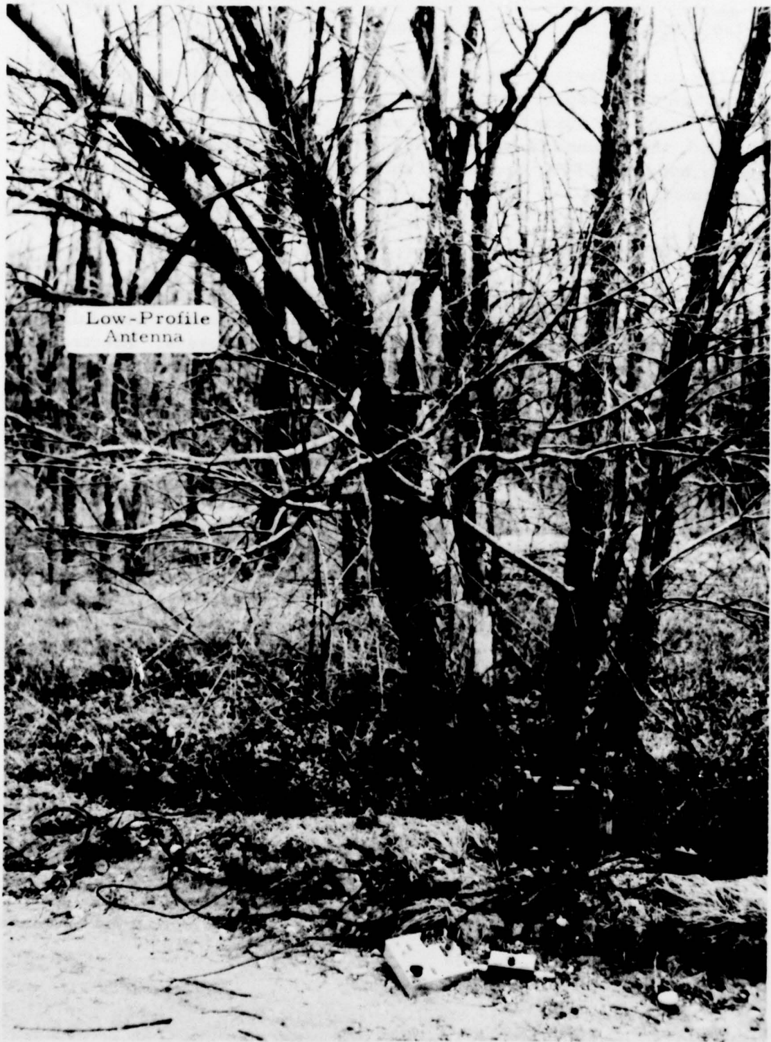
Fig. 14. Low-profile, remote-tuned dipole deployed in a tree.
