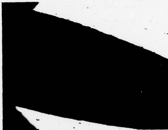
FIG. A4 Photograph of single Corning fiber cut at 75^\circ for three-fold collimation.
