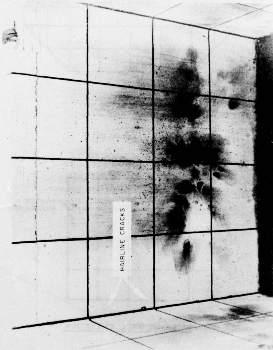
Fig 10 Post-test view of Cell No. 1 west wall (Test No. 2)
