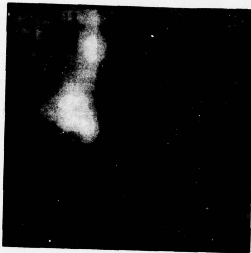
Fig. 6 Average high level extrema each point represents the total number of high level extrema within a 40x40 window centered at each point
