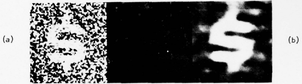
Figure 3 Computer Simulated Noisy Image (a) and Filtered Result (b). Signal and Noise Follow Model in Eq. 1; L=15 ; r(x,y) = 2/3 in Background and 4/5 in Foreground; t(x,y) is Uniformly Distributed Between 0.02 and 1.0. Filtering Process is as Shown in Figure 2.
