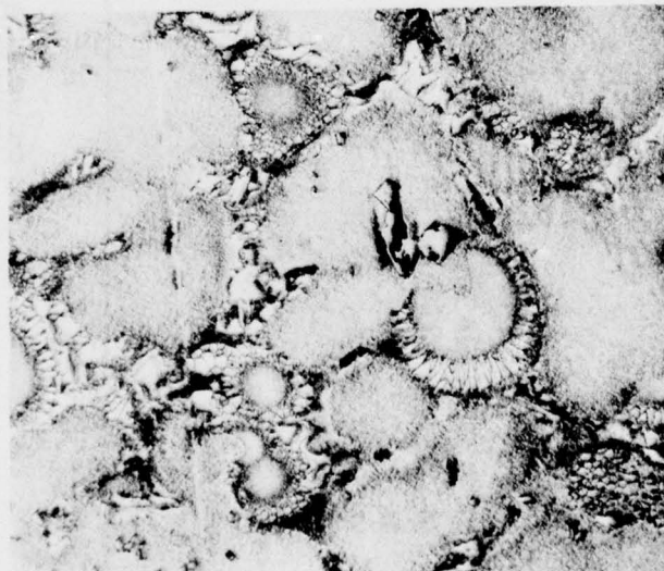
c) REFINED C 103 SHOWING CONVOLUTED, INTERLOCKING GRAIN BOUNDARIES AT 250X.
